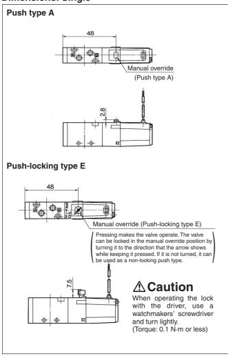
Note) Because the manual override unit protrudes, the manual override could activate unintentionally if the protrusion is touched or an object falls on it. Therefore, take the proper preventative measures.
