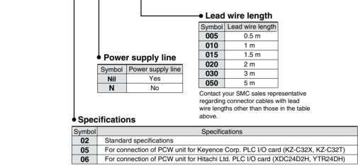
Note) When using a PCW unit equipped with Fujitsu FCN connector, contact your SMC sales representative as the connector cable is different.
