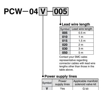
Refer to page 55 and "Best Pneumatics Vol. 1" for details regarding applicable manifold solenoid valves.
