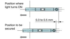
To set the detection point of the second point (and subsequent points), you will be required to prepare a new switch and set it from step 1.
