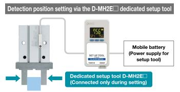
When there is no IO-Link master, the D-MH2ED dedicated setup tool can be used to set the detection position. As the tool is powered by a mobile battery, setting can be performed from any location. \* Does not include the mobile battery or USB-C cable
