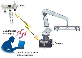
Can be introduced by OPC UA or the wireless system without connecting to a PLC or changing the program. Modular type F.R.L combination can be connected.
