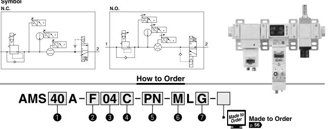
X101 Without residual pressure relief 3-port solenoid valve X102 Without standby regulator
