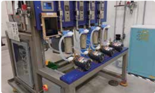
Pump assessments (endurance testing)
