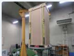
Transportation vibration testing
