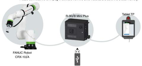
USB memory (Saved copy of FANUC CRX plug-in software)
