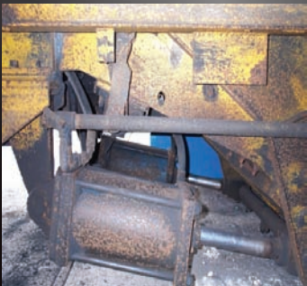
Coal wagon dump doors
