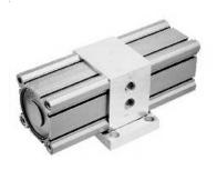
This 2:1 ratio air-to-air booster is small and self-contained and incorporates integral valve components to reciprocate. It was developed to amplify inadequate air pressure since doubling the input pressure can increase the output force of a cylinder where space constraints exist.
