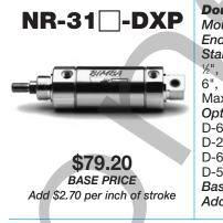
Adder Per Inch of Stroke: .15 **Double Acting** – Universal Mounting Type – Pivot or Double End – Air Return Standard Stroke Lengths: ½", 1", 1½", 2", 2½", 3", 4", 5", 6", 7", 8", 9", 10", 11", 12" Maximum Stroke 24" Optional Accessories: D-615 Mounting Bracket D-231-3 Rod Clevis D-620 Pivot Bracket D-508 Mounting Nut Base Weight: 1.62 Adder Per Inch of Stoke: .15
