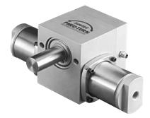
The Bimba Pneu-Turn® position feedback rotary actuator ( PTF ) provides continuous shaft position sensing. Standard features include shaft ball bearings and the elimination of mid-rotational backlash. Use the Bimba PTF in conjunction with Bimba's Pneumatic Control System ( PCS ) to achieve rotary shaft positioning accuracy within  $\pm 0.5^{\circ}$ .
