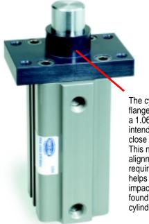
The cylinder mounting flange is designed with a 1.062" diameter hub intended to mate with a close fitting pilot hole. This not only aids alignment and location requirements, but also helps to withstand the impact loads commonly found in conveyor stop cylinder applications.
