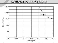
\* When an actuator is operated under conditions that exceed the lines on the graph above, be sure to use a regenerative absorption unit.
