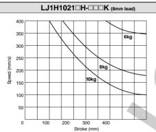
When an actuator is operated under conditions that exceed the lines on the graph above, be sure to use a regenerative absorption unit.
