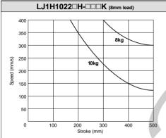
\* When an actuator is operated under conditions that exceed the lines on the graph above, be sure to use a regenerative absorption unit.
