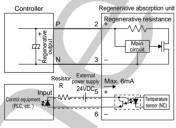
Note) Select 6mA or less for resistor R after confirming the input capacity of the control equipment.
