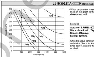
\* When an actuator is operated with conditions that exceed the lines on the graph to the left, be sure to use a regenerative absorption unit.
