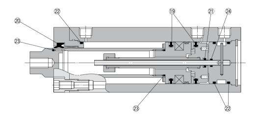
\* The numbers are the same as the "Construction" of the Best Pneumatics No.3 Series RZQ.
