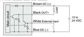
Max. applied voltage: 28 V, Max. load current: 80 mA, Internal voltage drop: 1 V or less External input: input voltage 0.4 V or less (reed or solid state input) for 30 msec. or longer
