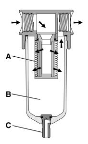
The contaminated air enters the element interior and is forced through a thick membrane (A) of "borosilicate" glass fibers coated with epoxy. Flow then passes through the element, and at this stage 99.97% of the sub micronic particles have been removed from the air stream. The tiny droplets coalesce together and are collected from the filter element by the outer drain layer.
