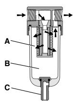
The contaminated air enters the element interior and is forced through a thick membrane (A) of "borosilicate" glass fibers coated with epoxy. Flow then passes through the element, and at this stage 99.97% of the sub micronic particles have been removed from the air stream. The tiny droplets coalesce together and are collected from the filter element by the outer drain layer.
